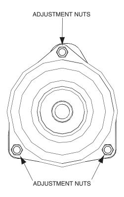
Figure 6-12. Clutch Air Gap Adjustment
